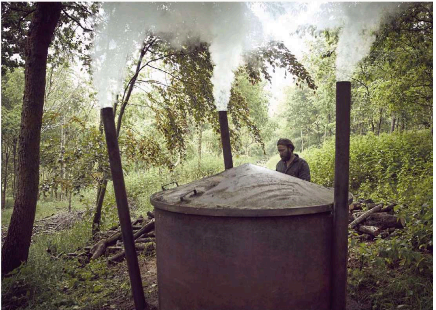
ABOVE A modern steel kiln has made the traditional charcoal-burning process slightly easier than it was years ago, but Ben still has to rely on the weather, condition of the wood and soil type to produce a good yield
